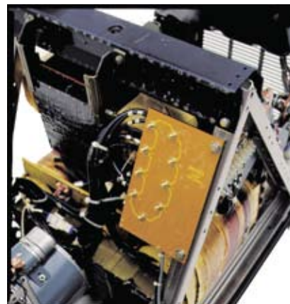
Coated Power Components & Panels
