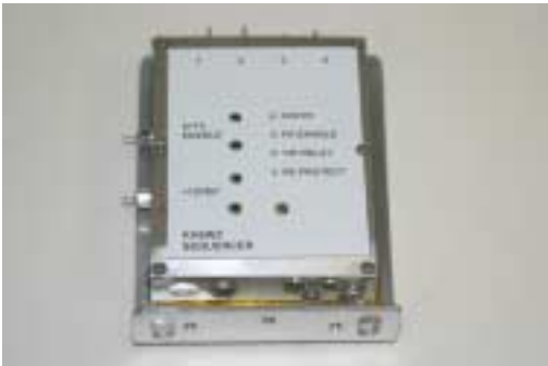
IMG_2355.jpg Sequencer with cover in place
