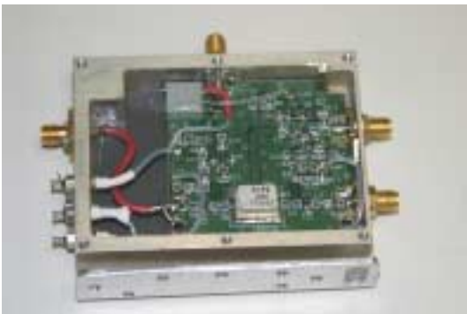
IMG_2353.jpg 3GHz Up/Down converter/mixer unit in a similar surplus milled case
