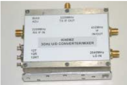
IMG_2353.jpg 3GHz Up/Down converter/mixer unit in a similar surplus milled case
