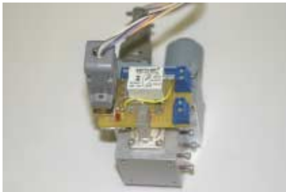
IMG_2359.jpg WR-42 T/R relay board. The "sub-relay" is a
