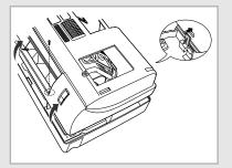
4 Remove screws (4EA) securing the front panel, then detach the front panel from the indoor unit.
