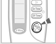
2 If the sign is not displayed at the top of the remote control, press the MODE button on the remote control one or more times until it appears.
