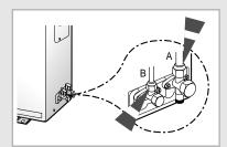
Before completing the installation (insulation of the cables, hose and piping and fixing of the indoor unit to the installation plate), you must check that there are no gas leaks.
