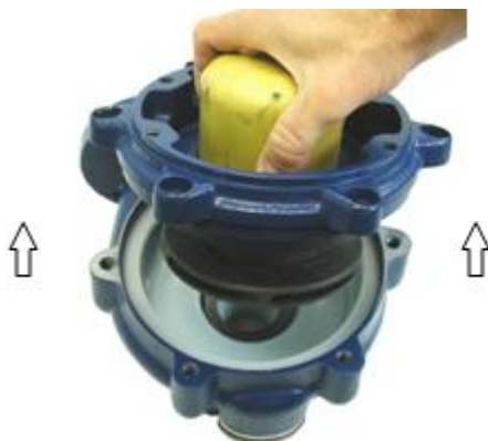
Figure 7: Open wet end.
