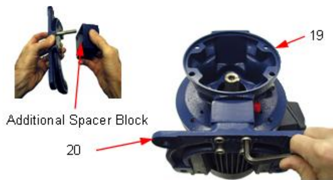
Figure 37: Installing Pump Riser
