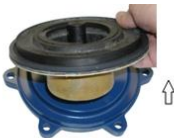
Figure 9: Remove containment shell
