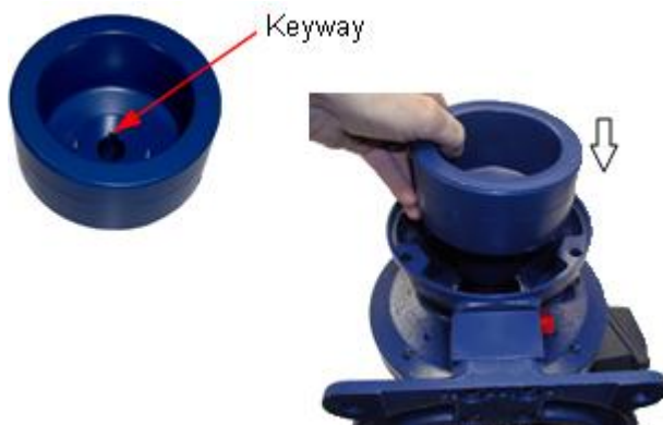
Figure 38: Installing Outer Magnet Assembly
