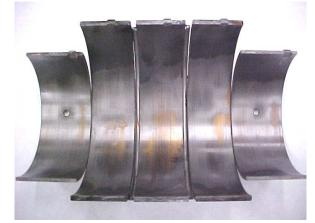
Faint copper showing on main & rod bearings in the loaded area is another indication of dust out.
