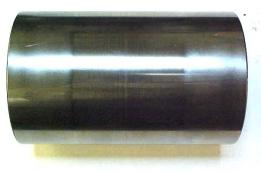
Cloudy piston pin surface in the area that the piston dome rides is also an indication that abrasive material has entered the engine.
