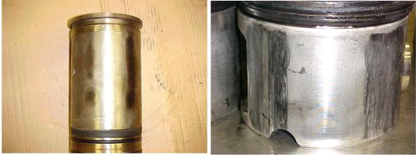
Quarter point scuffing is an assembly error and is not a warrantable failure.
