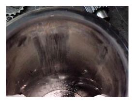
Fire ring scuff will show near the top of the liner at the ring reversal area. This is the hottest part of the combustion process.
