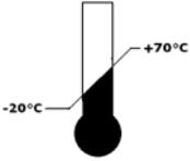
Symbol for "temperature limitation." The upper and lower temperature limits will be indicated on either side of the symbol
