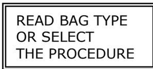
This function allows to enter the menu to select the desired procedure. The procedure can be selected manually by pressing key
