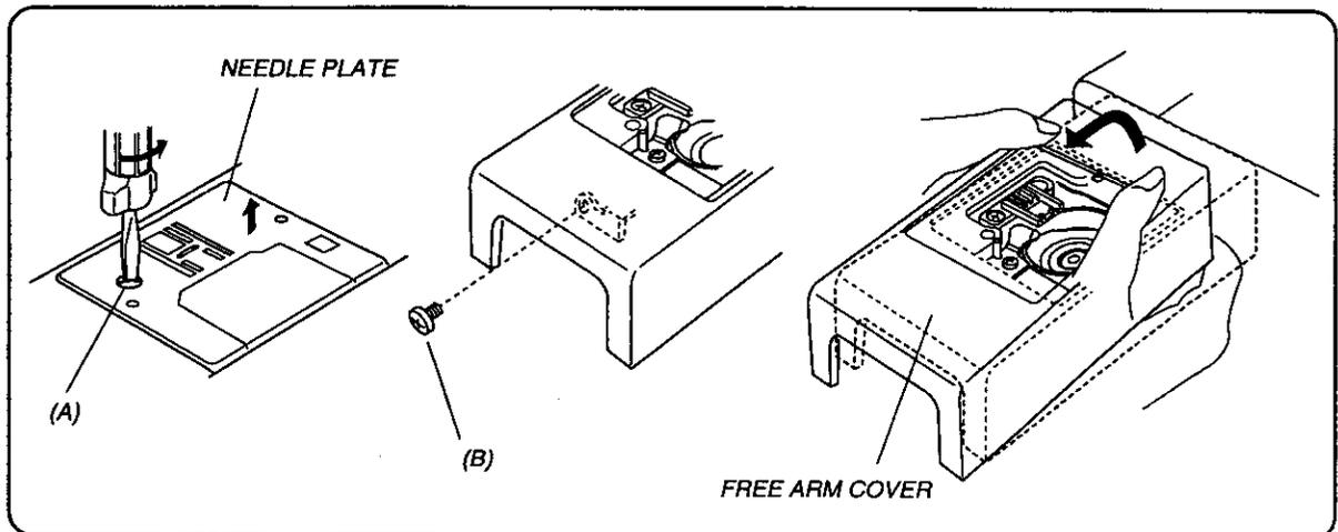
1. REMOVE THE SETSCREW (A) AND THE NEEDLE PLATE.
