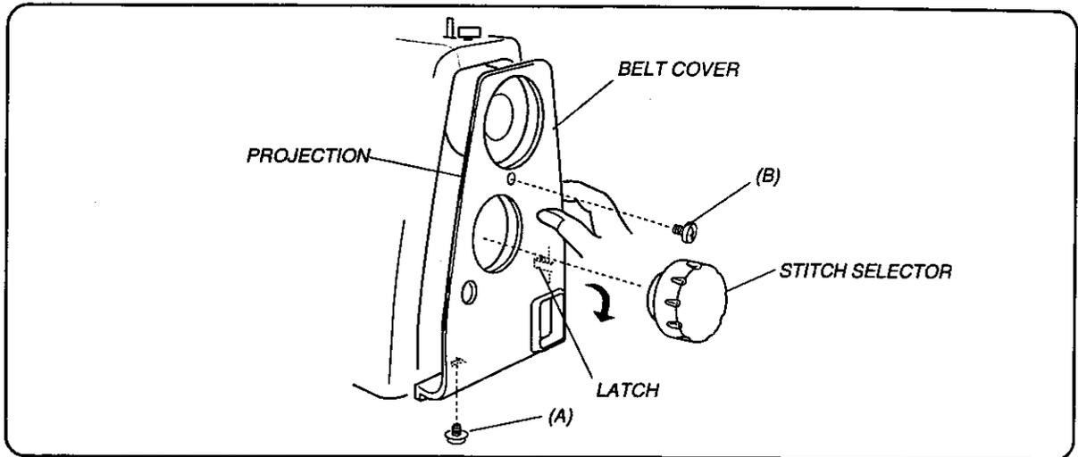
PULL OUT THE STITCH SELECTOR. LOOSEN THE SETSCREW (A) AND REMOVE THE SETSCREW (B). PULL THE RIGHT SIDE OF BELT COVER IN THE DIRECTION OF THE ARROW, AS ILLUSTRATED AND TAKE THE LATCH OFF, AND THEN REMOVE THE BELT COVER.
