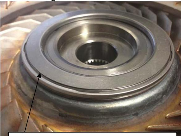
Larger diameter thinner bearing placed on turbine (this side up)
