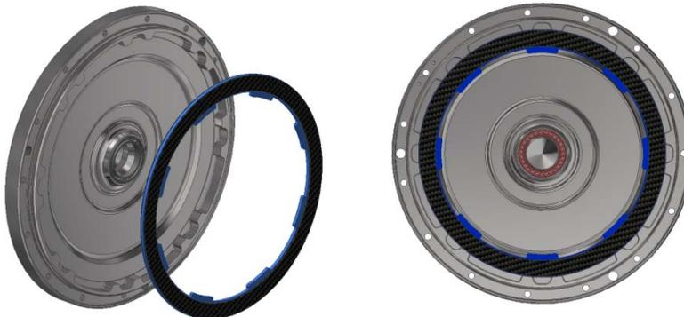
5. Next place single-sided friction into front. The single-sided must be placed on top of double-sided friction and must be placed with friction side up.
