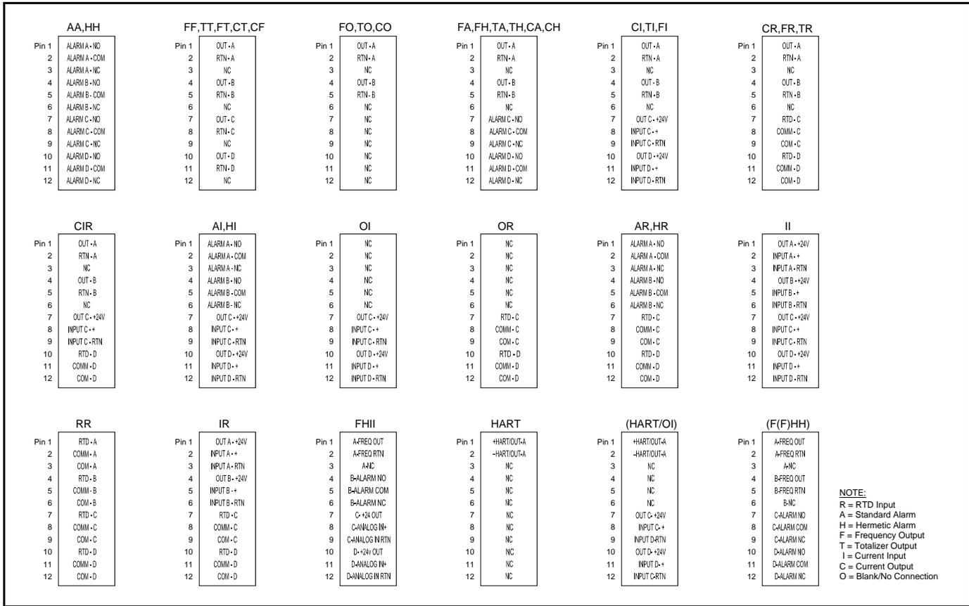
Figure 1-11: Option Card Connection Labels (ref. dwg #442-615)
