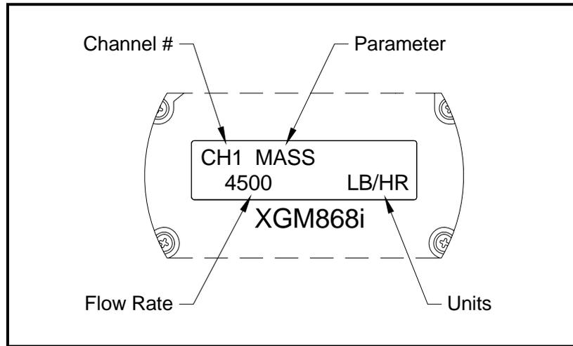
**Figure 3-1: A Typical LCD Flow Rate Display**
