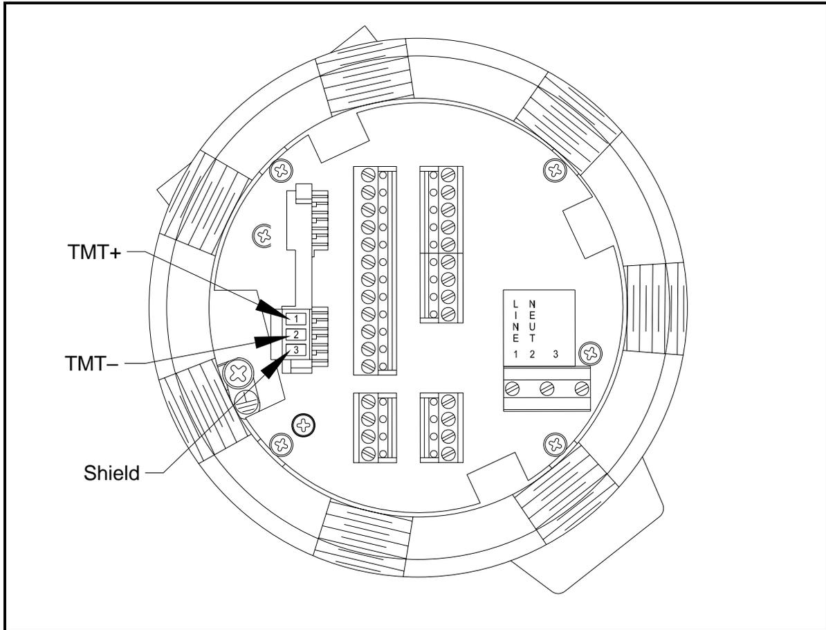
**Figure 1-7: The RS485 MODBUS Terminal Block Connector**
