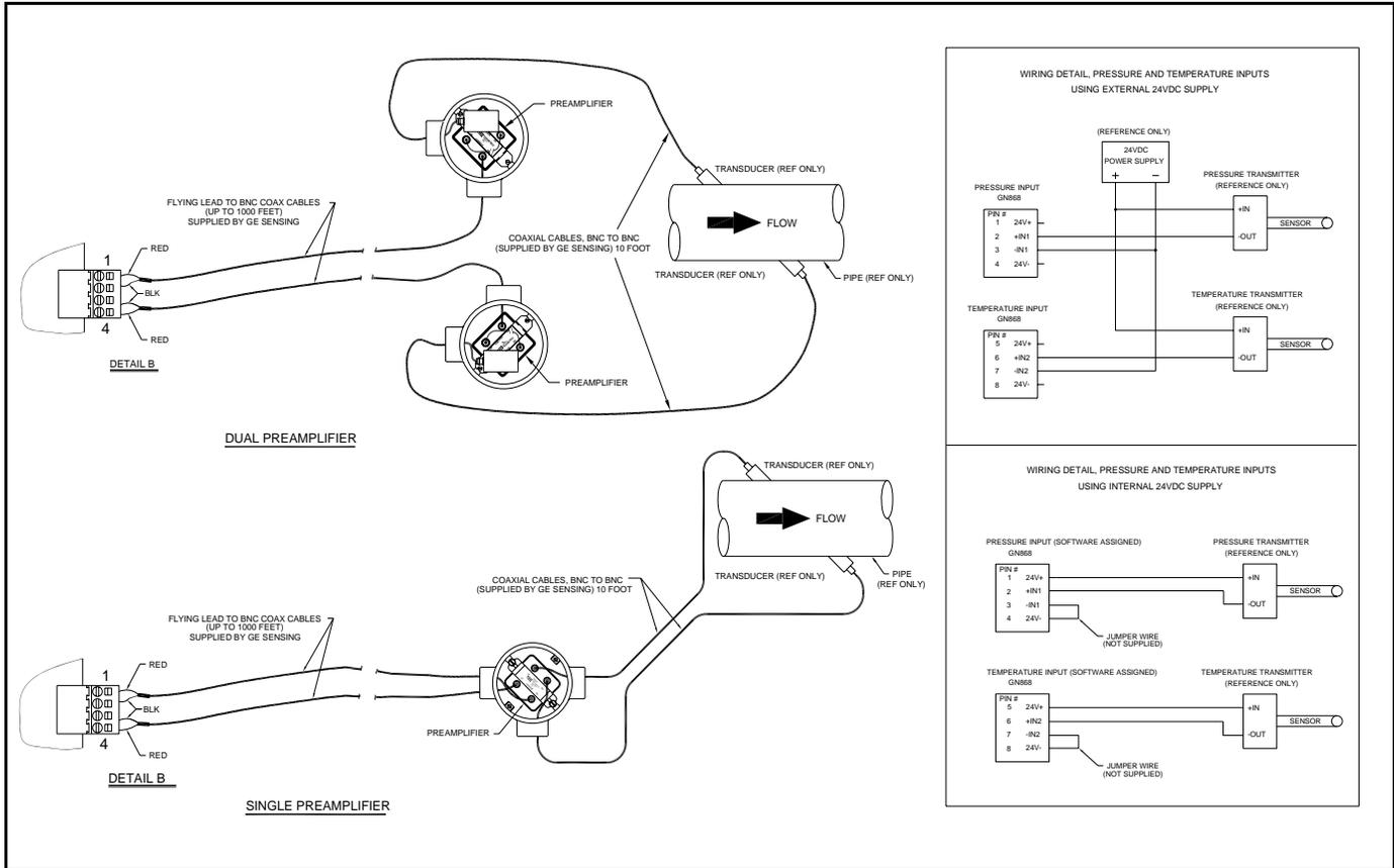
Figure 1-12: Transducer Wiring Diagram (ref. dwg #702-213)
