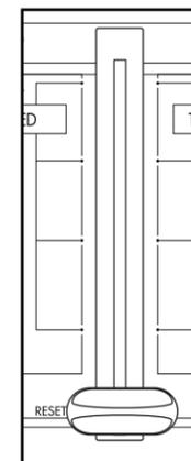
To stop the walking belt, step onto the foot rails and move the speed control to the RESET position.
