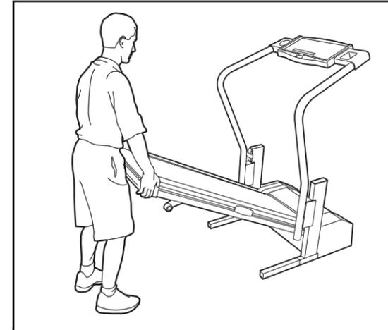
2. Move your right hand to the position shown at the right, and hold the treadmill firmly. Raise the treadmill until the storage latch locks over the frame guide. **Make sure that the storage latch closes fully over the frame guide.**
