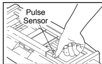
Next, raise your thumb slightly until the heart-shaped indicator in the PULSE display flashes **steadily**. Hold your thumb at this level.
