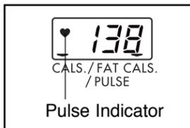
After a few seconds, three dashes will appear in the display and your pulse will be shown. Hold your thumb on the sensor for another 15 seconds for the most accurate reading.
