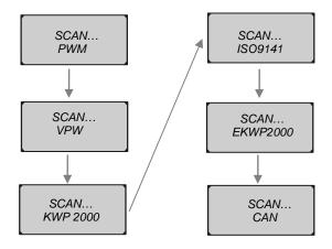
• Not all the above messages will be displayed unless protocol of the vehicle being tested is the last one—the CAN protocol.
