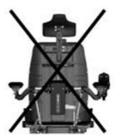
The wheelchair must NOT be fastened by securing it to any part of the seat.
