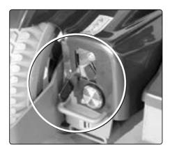
Brake release lever with safety catch
