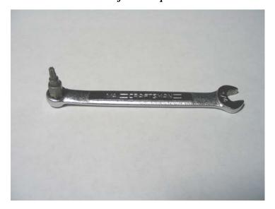
After you "break free" the small Torx bolts, use a ¼ inch ratchet with a ¼ inch socket and insert the Torx bit into the ¼ inch socket. This will "speed up" the removal of the small Torx bolts that hold the tre crossover lines to the fuel injector rails.
