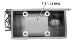
(4) Remove the set screw on the sirocco fan and the two motor set screws to remove the sirocco fan and fan motor. (Fig. 6)
