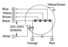
Measure the resistance between the terminals with a tester.
