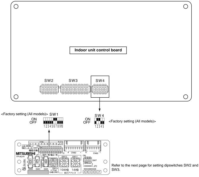
1) When using an ME remote controller, set the address with the rotary switches (SW11, SW12).
