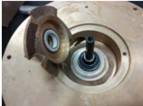
Ceramic seal pressed into propeller
