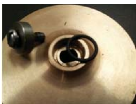
Large o-ring in top of impeller
