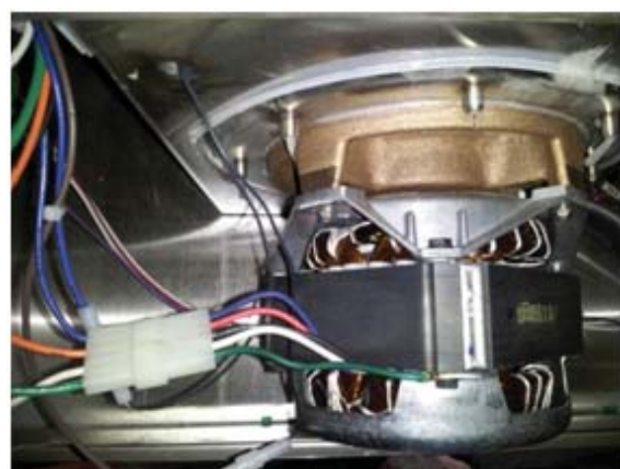
Pump motor, black wires to float can be seen upper left
