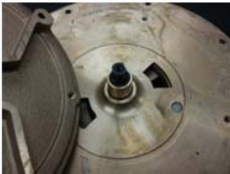
Suction plate, housing removed
