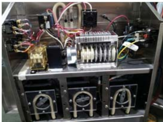
Showing detergent, rinse, sanitizer internal chemical pumps
