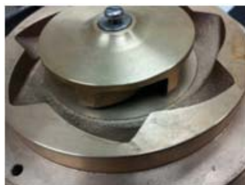
Diffuser removed, centrifugal Impeller
