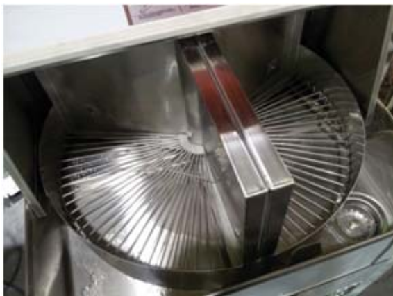
Carousel is rotated manually, shows correct position for cycle
