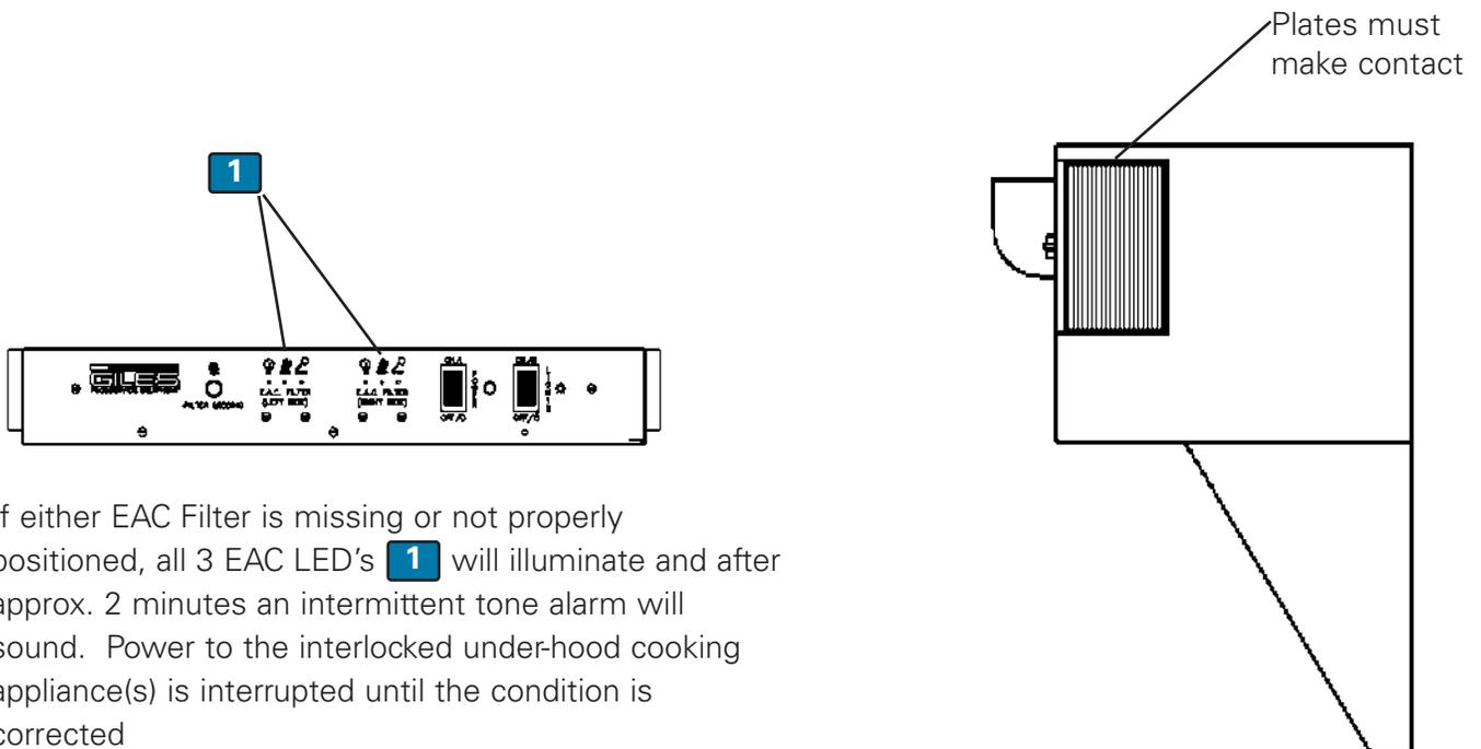
If either EAC Filter is missing or not properly positioned, all 3 EAC LED's **1** will illuminate and after approx. 2 minutes an intermittent tone alarm will sound. Power to the interlocked under-hood cooking appliance(s) is interrupted until the condition is corrected
