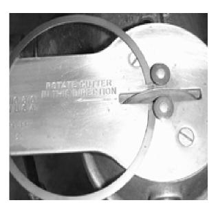
good chance of chipping the ring face which will cause engine damage while running. Remove burrs from rings after grinding or filing, then thoroughly clean.
