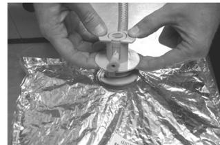
4. Push QCD plunger into bag spout until plunger top is flush with top of QCD. A "click" will be heard when it is fully inserted.
