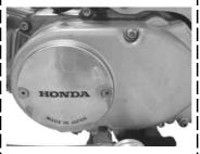
Inject engine oil to the level specified by the relevant clutch kit.
