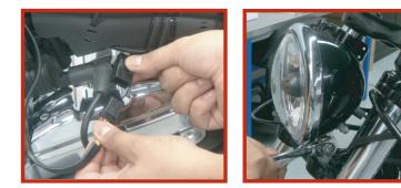
4. Remove the stock bezel trim using a phillips screwdriver. Keep the headlight assembly in tact since the RSD bezel can installed now.
