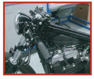
3. With the tank removed, locate the headlight wiring harness connector and disconnect. Note: Motorcycle models will vary so refer to the HD service manual for your specific model. With the harness unplugged, remove the headlight.
