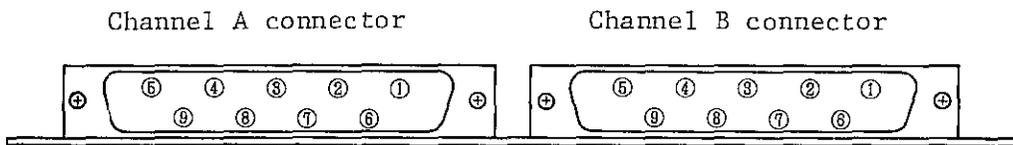
Fig.4-2. Connector pin configuration
