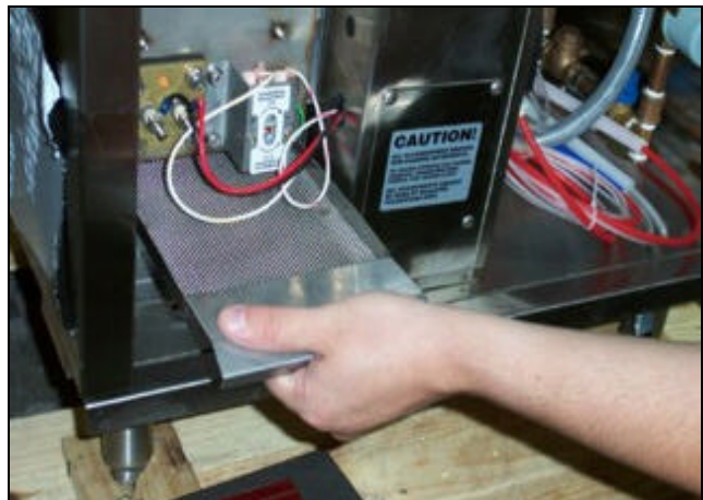
Removing the lower strainer.
