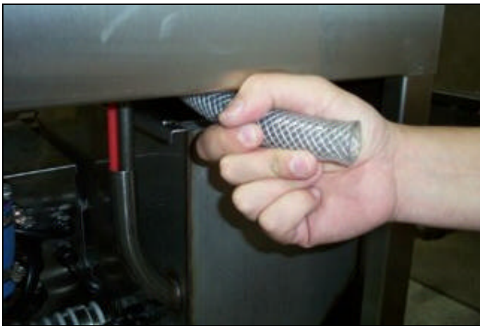
Pulling the discharge hose out.
