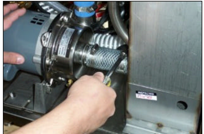
Loosening the suction hose clamps.
