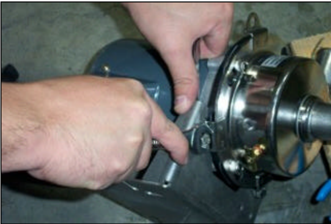
Removing the mounting bracket.
