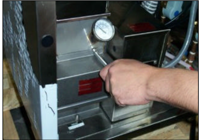
Removing the heater cover.
