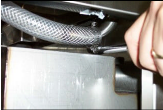
Loosening the discharge hose clamp.
