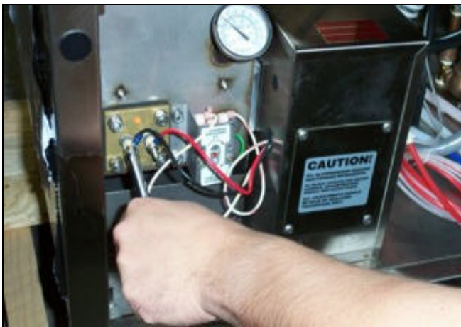
Removing the heater nuts.
