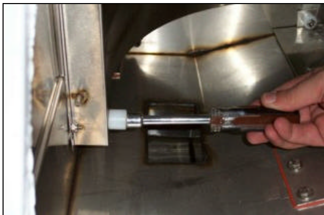
Loosening the roller locknut.
