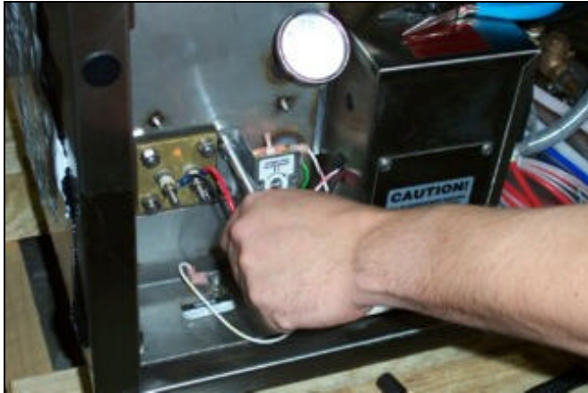
Removing the thermostat bracket mounting nuts.
