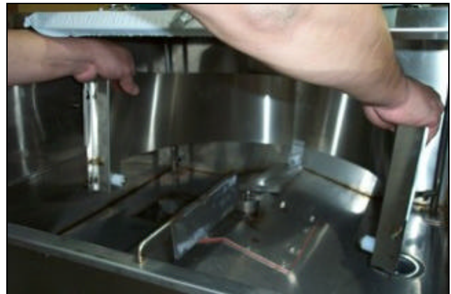
Remving the rack wrap.
