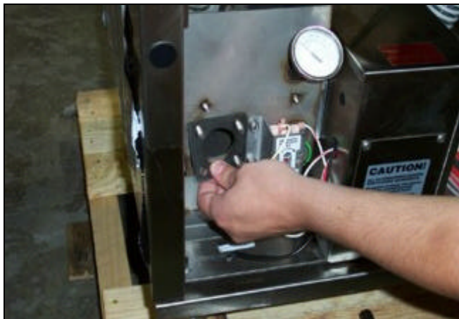
Removing the heater gasket
