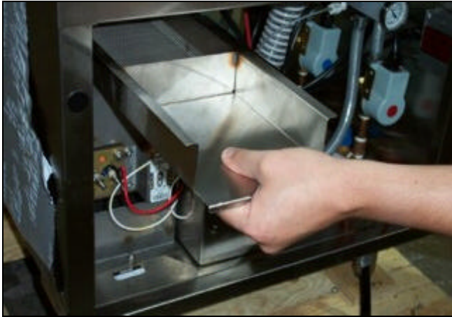
Removing upper (wash) strainer.
