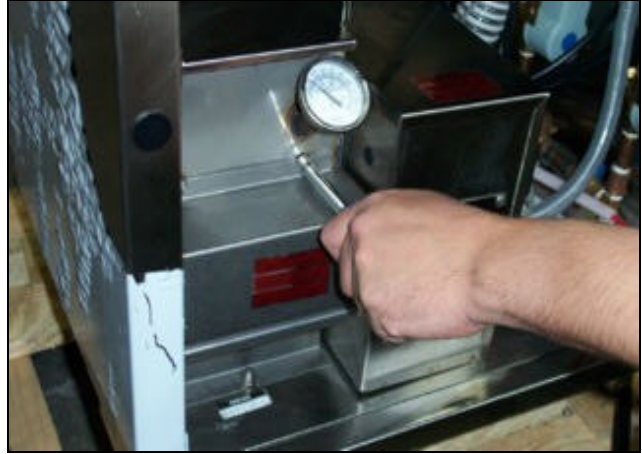
Removing the heater cover.
