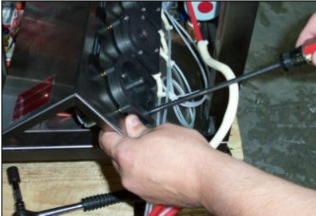
Removing the motor mounting screws.
