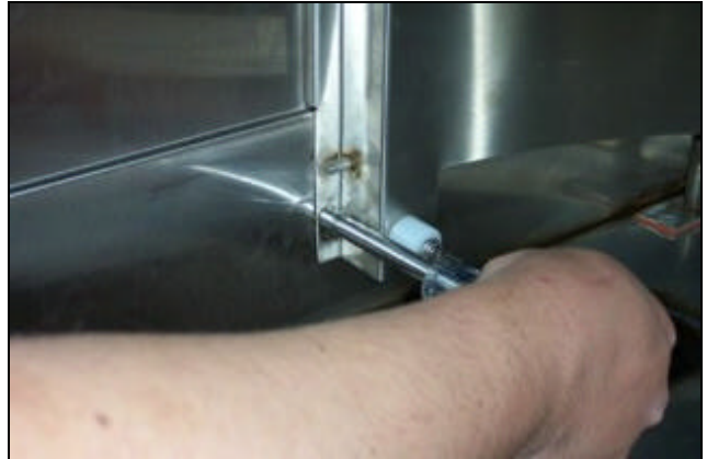
Remvoing the locknuts.
