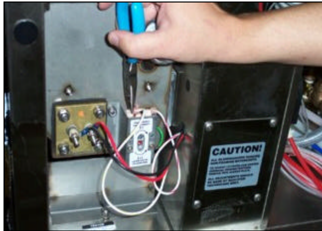
Removing the terminals.
