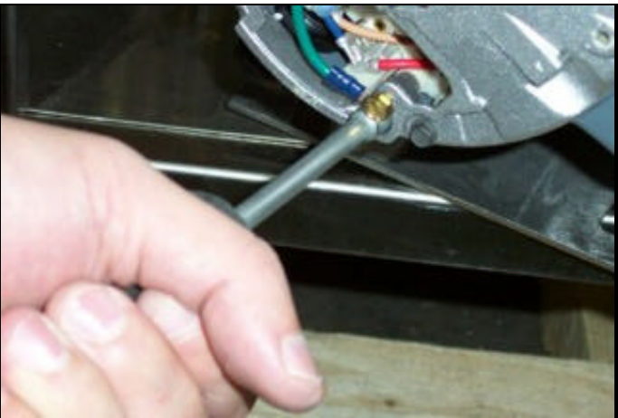
Removing the grounding screw.
