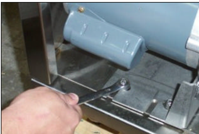
Removing the assembly mounting nuts.
