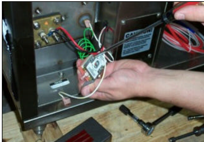
Separating the thermostat from the bracket.
