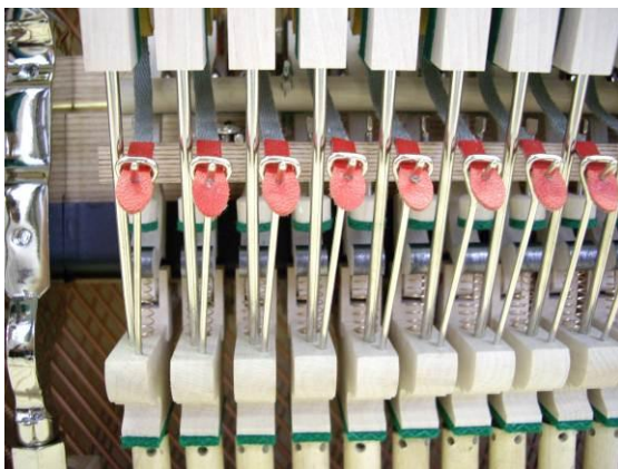
aligned bridle strap-tapes: Make sure 1mm space is between back check wire and bridle strap.
