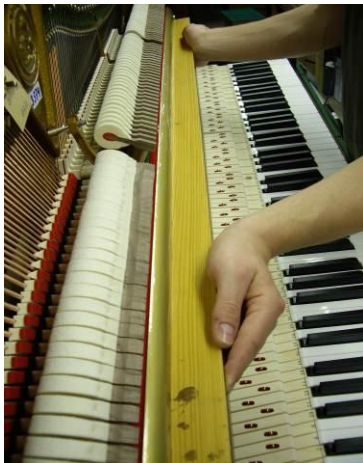
check hammer-rest rail with straight edge
