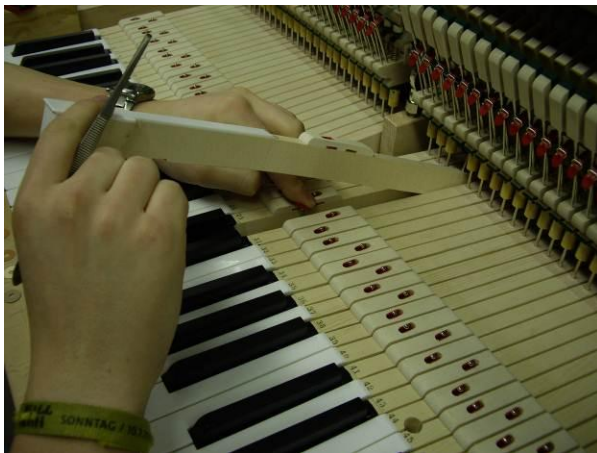
to insert or remove the different paper washers at the balance pin
