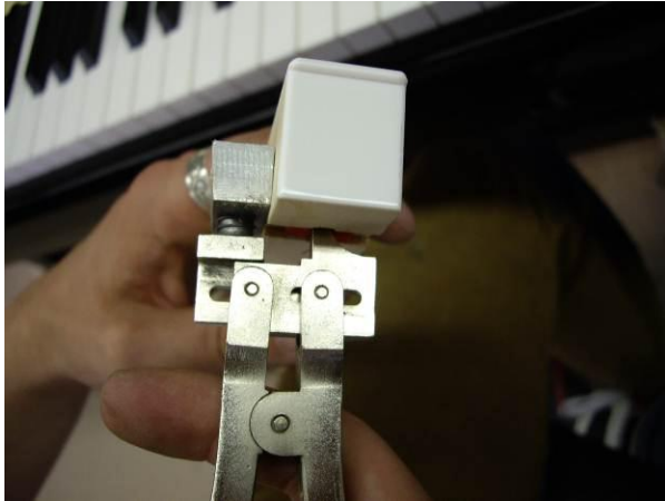
compress the front key bushing with the key-easing pliers
