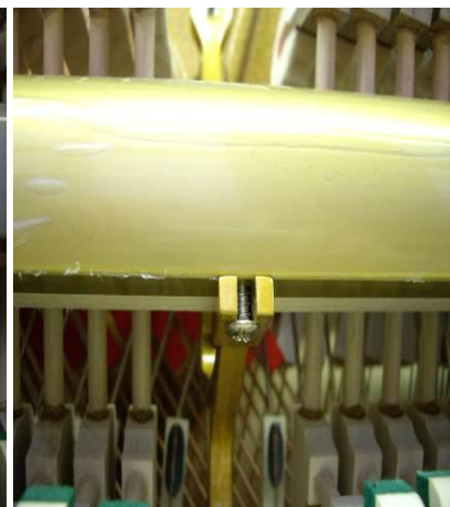
screw of angle bracket unscrew the screws for adjustment of hammer-rest rail
