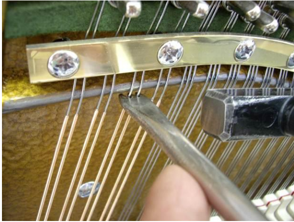
adjust gently tap the string spacing
