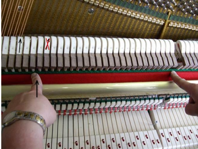
Push the hammer-rest rail with fingers to the strings to check lateral movement of hammer due to flange.
