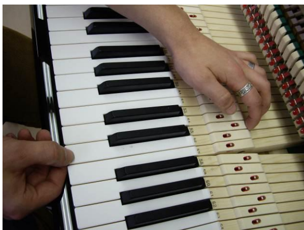
check the lateral movement at the front pin with key at rest
