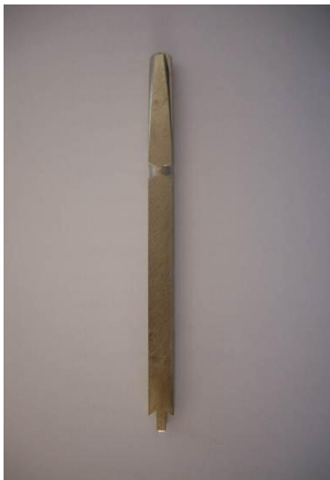
key bushing tightener, tap gently
