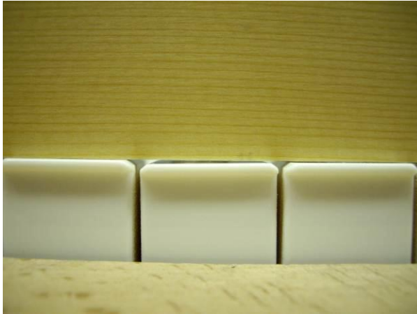
middle key surface not parallel to others
