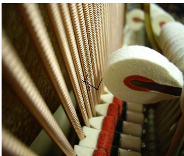
Let-off distance between hammer and strings
