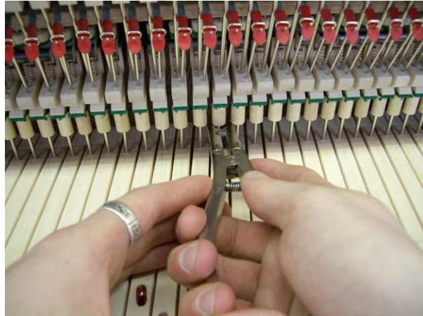
adjust the capstans centrally under the wippen heel
