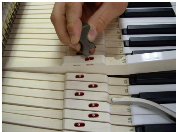
needle the balance rail bushing
