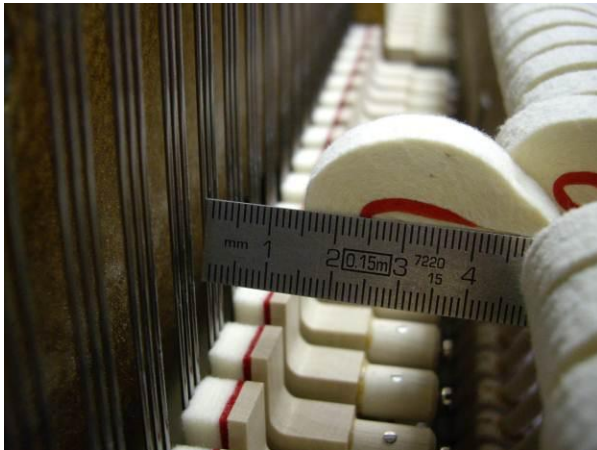
checked key 15mm before the strings
