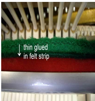
Insert and glue a thin felt strip
