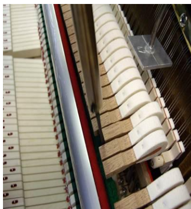
iron the rest rail felt by using a hot tool
