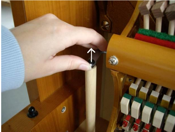
raise up the half-blow arm to release the pedal-rod
