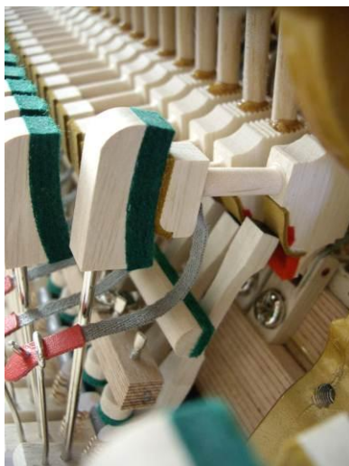
left picture: position of the back check when hammer is caught
