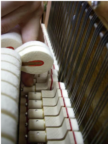
2mm distance between damper and damper stop rail (when key is depressed)
