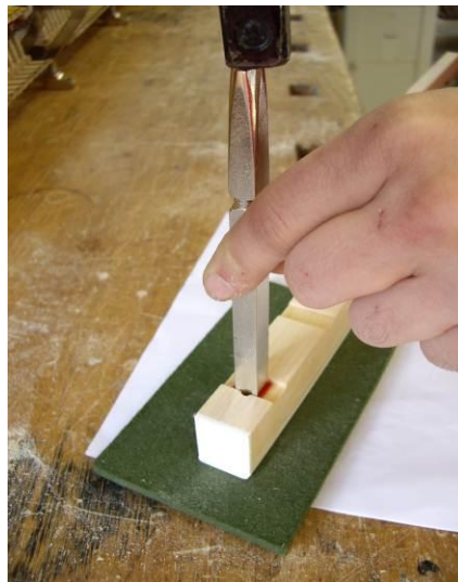
key bushing tightener, tap gently
