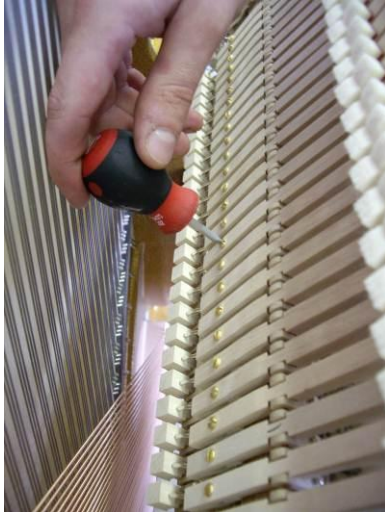
adjust the damper-lift with the damper-lift regulating-screw
