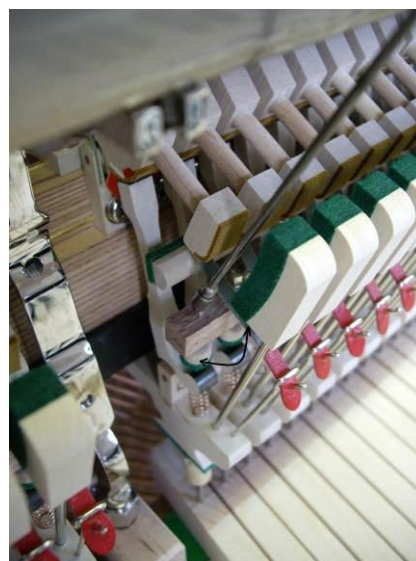
Turn the regulating screw with the jack button regulating tool.
