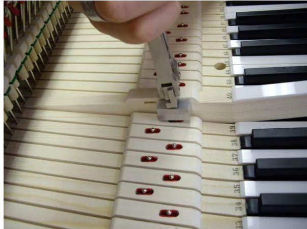
compress the balance rail bushing
