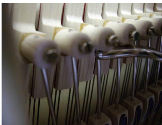
bend the damper wires for parallel adjustment to the strings
