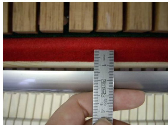
bridle-tapes follow half-blow-rest rail after moving 13 -15mm
