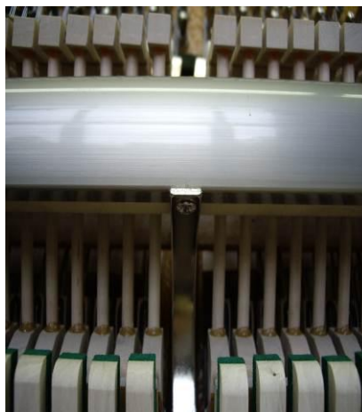
screw of angle bracket unscrew the screws for adjustment of hammer-rest rail
