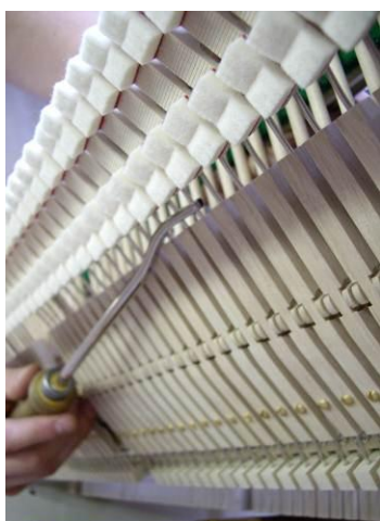
bending the damper wire for adjustment parallel to the strings
