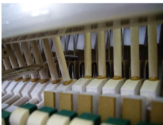
bend the damper wires for parallel adjustment to the strings
