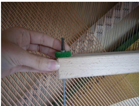
picture nr.2: adjust screw of mute rail
