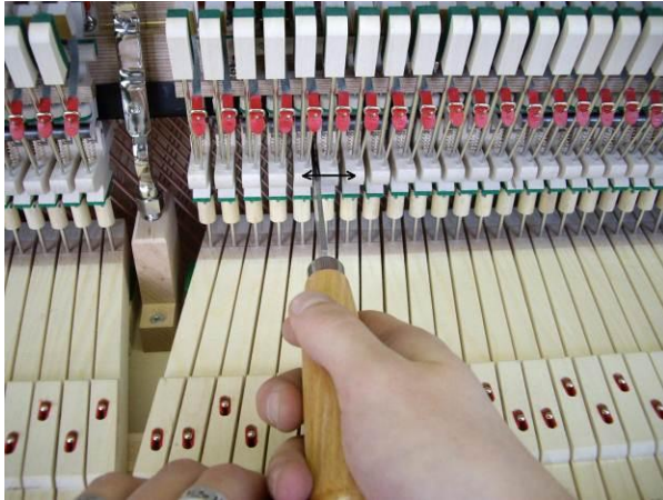
adjust the distances between the wippen heels the flange spacer
