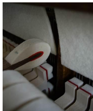
picture nr. 4:hammer hit the muting-felt at this level
