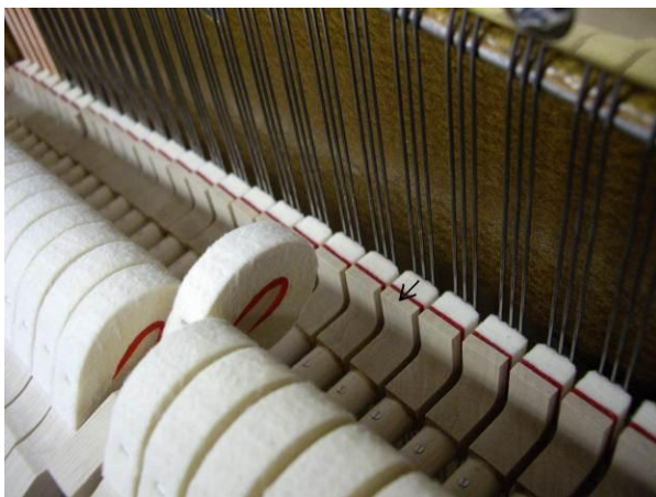
damper begins to lift at this moment
