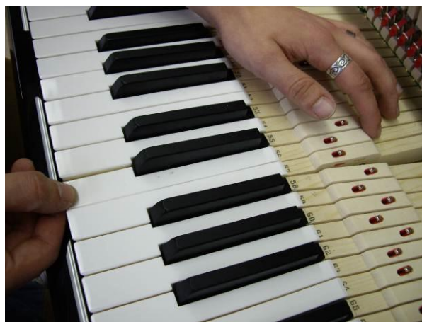
check the lateral movement at the front pin with depressed key
