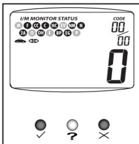
Monitor icons on the LCD display. A **blinking** Monitor icon means the Monitor has not yet run and finished its diagnostic self-testing. All Monitor icons that are **solid** have completed their diagnostic self-testing.
