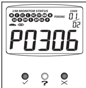
**MONITOR STATUS** - If the Code Reader's LCD display shows a zero (indicating there are no DTCs present in the vehicle's computer), but the yellow LED is lit, it indicates a "Monitor Has Not Run" status. This means that some of the Monitors on the vehicle have not yet finished their diagnostic self-testing. This condition is confirmed by one or more **blinking**
