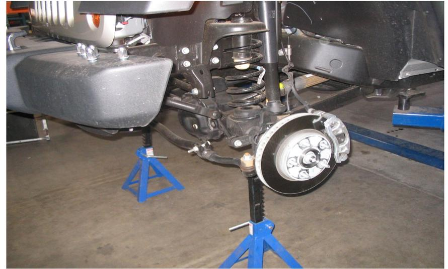
2. With the jack under the front axle, jack up the axle to remove the driver side and the passenger side wheels then disconnect the shock and sway bar end link on the driver side then the passenger side.
