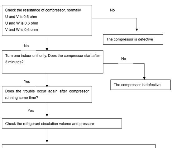
If refrigerant circulation volume and pressure is OK, change the outdoor main PCB.
