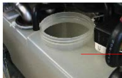
Disinfection solution tank with cover and fluid level sensor removed
