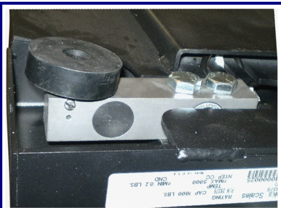
Example of Load Cell from a Mild Steel Scale
