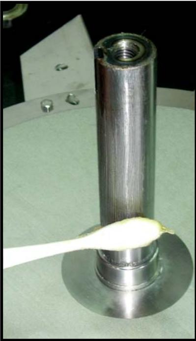
1. Apply axle grease to main shaft before installation.
