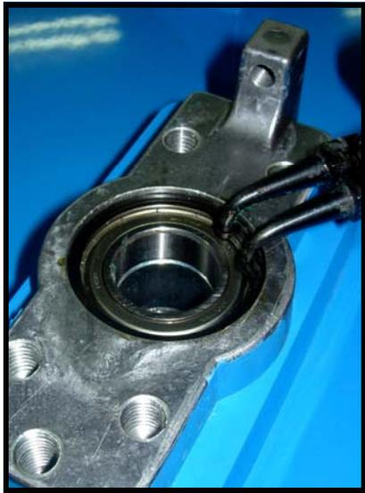
1. Remove C-clip from rear of aluminum housing
