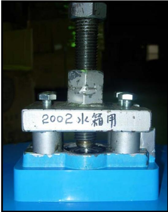
First, attach the FDF flywheel shaft puller to the rear of the SMC tank aluminum housing and tighten the four bolts as shown. Then, with a large open-end or crescent wrench, slowly turn the main puller bolt clock-wise until the flywheel is forced through the housing and out of the tank.
