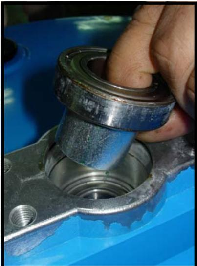
3. Remove Rear bearing and spacer
