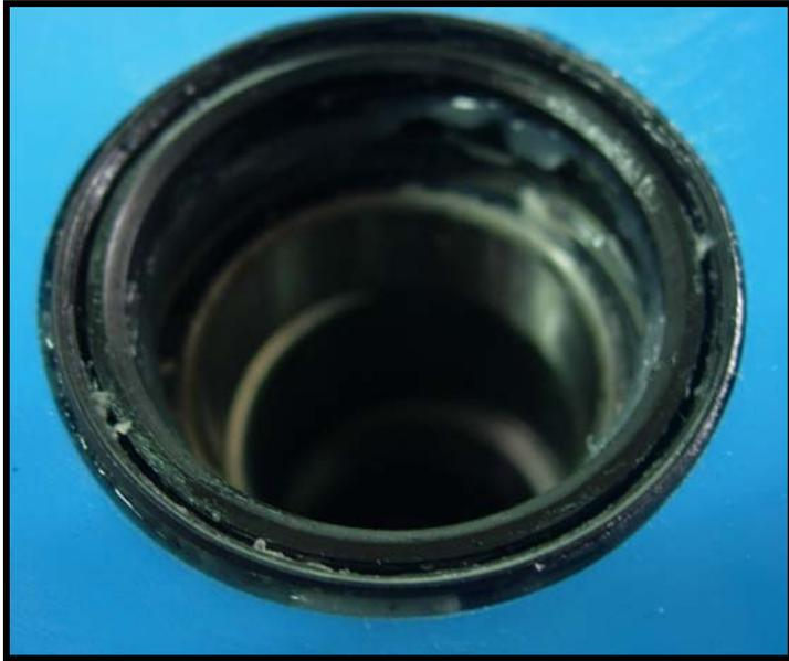
On the left is a healthy tank shaft seal, the silicone glue and packing grease maintain their original color. The integrity of this tank shaft seal has not been compromised. The bearings will show no sign of water damage and run smoothly. If there are no issues with the tank bearings, the bearings and tank shaft seal can be left in place and the tank re-assembled.
