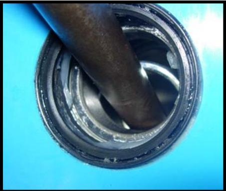
2. With small drift and hammer, lightly tap out and remove the rear bearing
