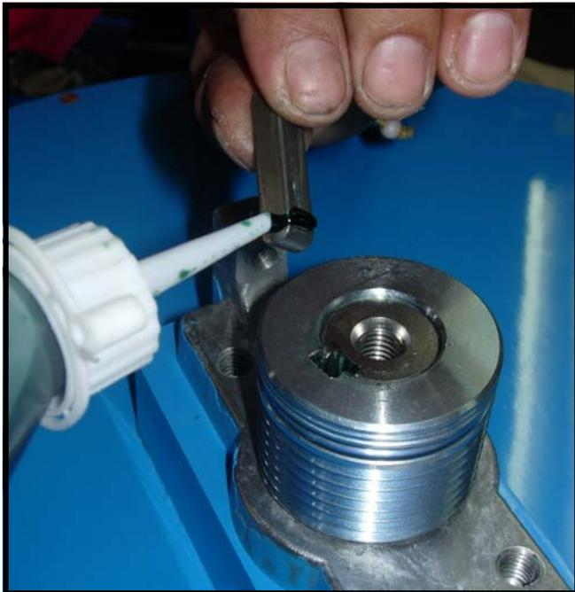
2. Apply thread locker to the keyway before knocking into place. Use a drift or heavy bladed screwdriver to drive the keyway into place as shown upper right.
