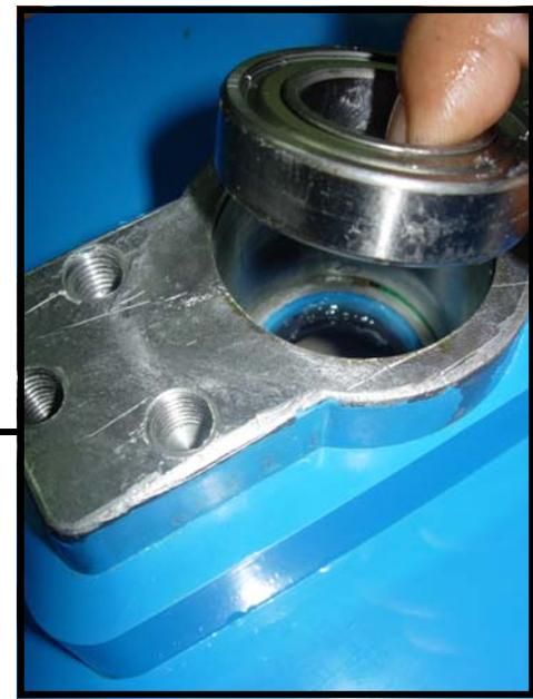
4. Tap out the front bearing and remove
