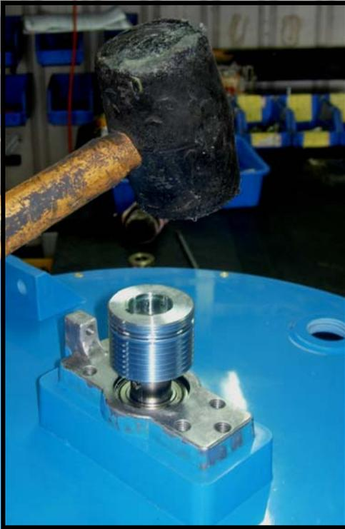
1. Reinstall the Small belt pulley onto the main-shaft. Remember to keep the keyway positions on the shaft and pulley lined up as you go.
