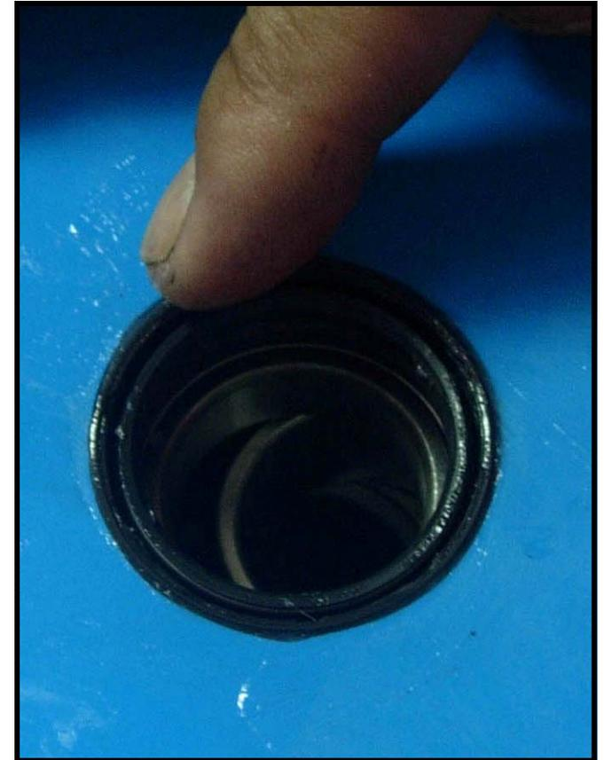
2. Apply silicone glue to the outside of the NBR tank seal prior to pressing the seal into the SMC tank back. Standard fish tank grade Silicone is required.
