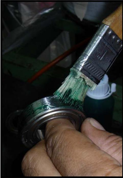
1. Clean inside of aluminum housing. Add thread locker to the outside of the bearing and to the inside of the aluminum housing where the two bearings will be located. Note that the service tech will be required to rig up a tool of some kind to tap the front tank bearing in. An example of the set up we use at the factory is shown below. A simple washer and metal spacer will also work. Check that the bearings are rotating smoothly once seated in the housing.
