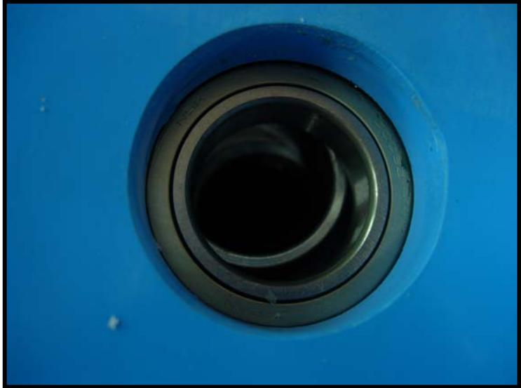
1. Carefully remove any residual matter (silicone glue or grease) from the SMC seal housing walls before pressing in the new seal housing.
