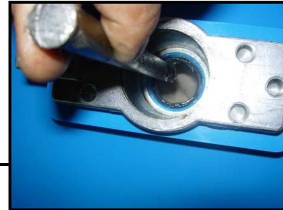
5. Lightly tap out the mainshaft seal and remove
