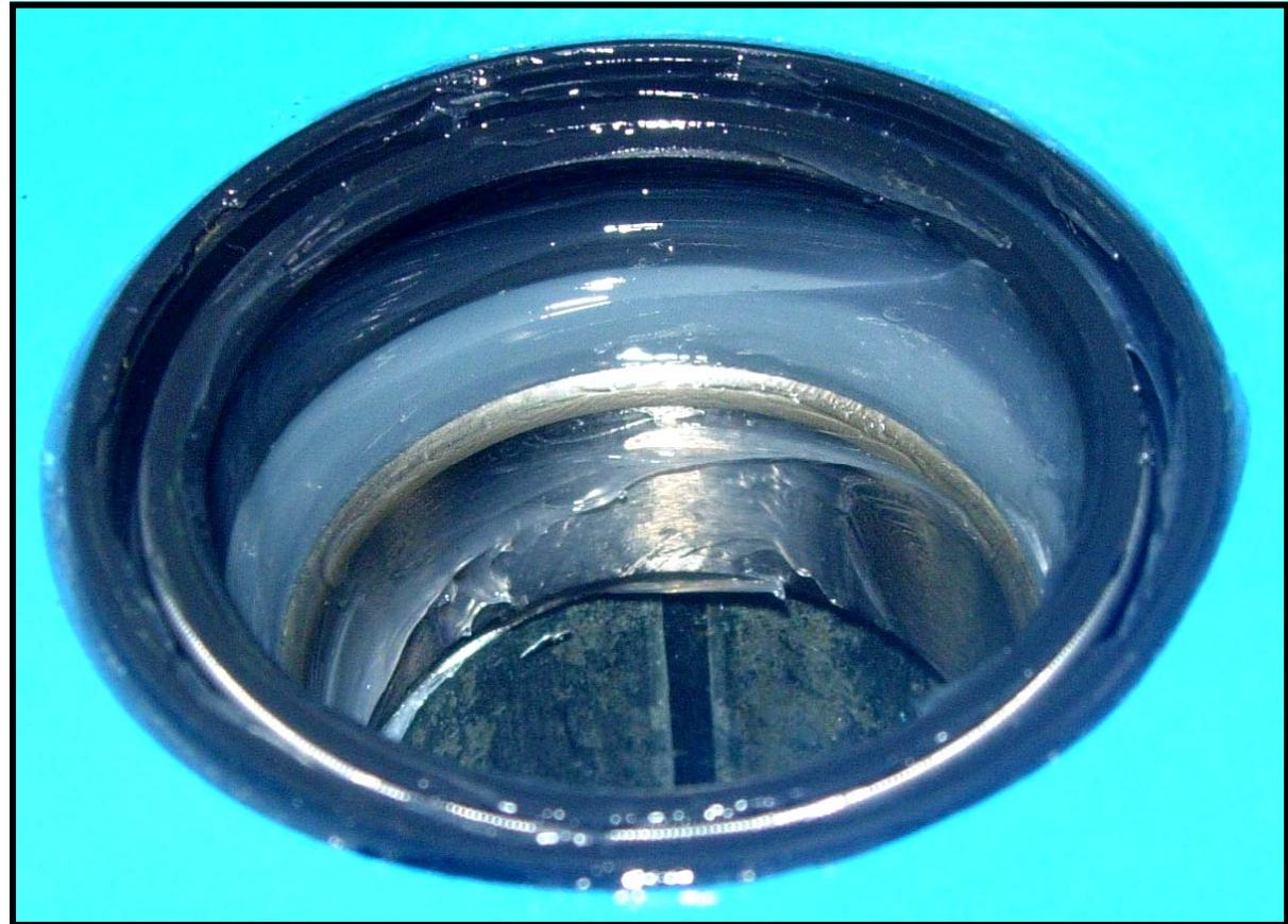
Apply a generous amount of Silicone grease (standard O-ring grease) to the inside of the seal and pack the area between the rear of the seal and the front bearing with a liberal amount of O-ring grease. Above right is an example of a properly prepared tank shaft seal .
