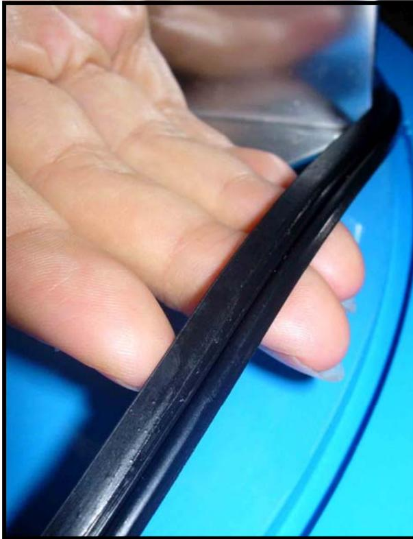
1. Lay the O-ring into the SMC O-ring groove, making sure it is flat and flush before securing the PC cover. An improperly laid and prepared O-ring will seep water over time. If the seal is excessively dry, then add a light coat of silicone grease.
