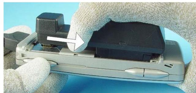
4.) When removing the Adapter, first release tension by pressing as shown in the picture.
