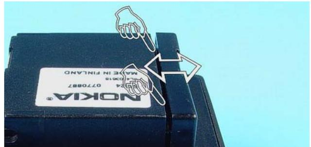
The Flash Adapter is equipped with a movable part, which is attached to the springs for fitting into the battery holder.
