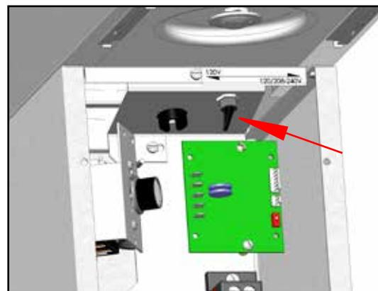
**FIG. 5-1 Dual Volt Switch Position**
