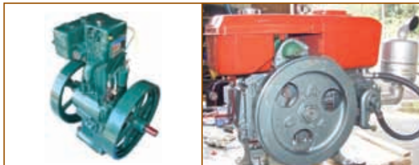
Lister (left) and Changfa (right) engines are typical of “historical-style” diesel engines.
