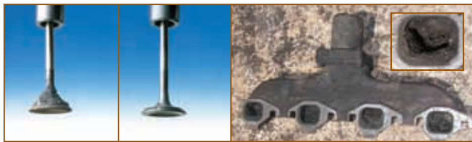
Carbon deposits on head of exhaust valve and inside exhaust manifold indicate incomplete combustion.
