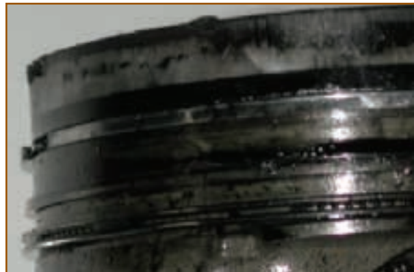
Partially burned fuel on the cylinder walls has caused the top piston ring to stick and completely malfunction.
