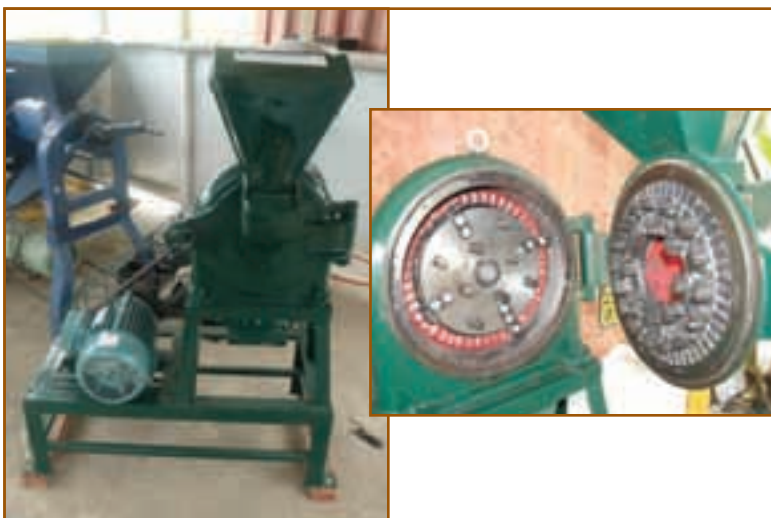
Small disk mill of the FFC range is powered by a 3kW motor.
