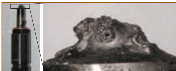
This multiport injector tip shows significant carbon buildup, which has a self-enforcing effect.
