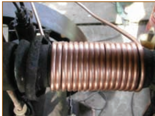
Copper tubing coiled around the exhaust of this Lister heats the fuel to 80–90°C before it is injected.
