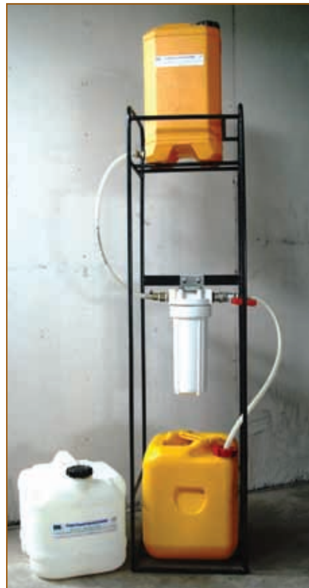
A simple gravity-filter system is a suitable option for filtering the low volumes of coconut oil produced by hand pressing.
