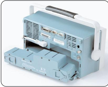
▶ *Battery pack being installed. The TDS3000B oscilloscope weighs only 4.5 kilograms with battery pack.*
