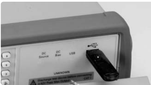
Figure 10. A USB memory device can be used to save set up states, data or graphs
