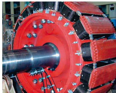
Salient-pole rotor, laminated, for piston compressor drive type DTKVY 2523-16WS
