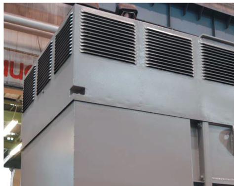
Open cooling circuit
