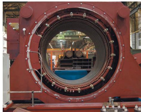
Stator for rolling mill drive, type DMMYZ 2246-6Y
