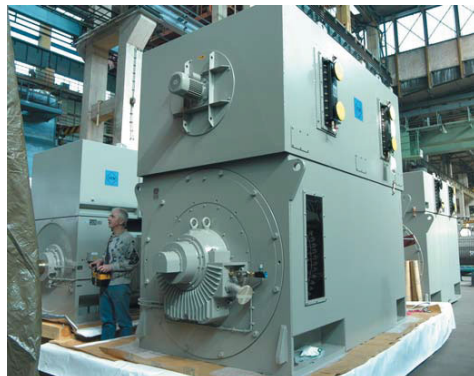
Synchronous motor for frequency converter operation, rolling mill drive, type DMMYZ 8044-6Y
