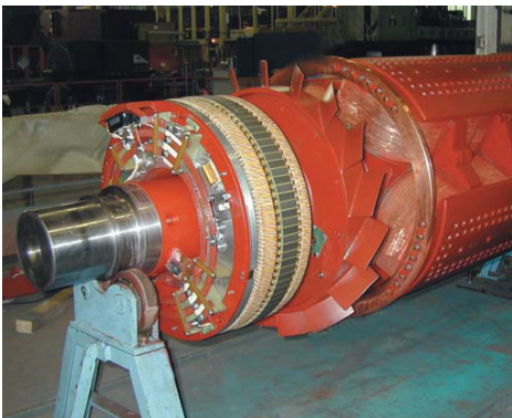
Salient-pole rotor with excitation machine
