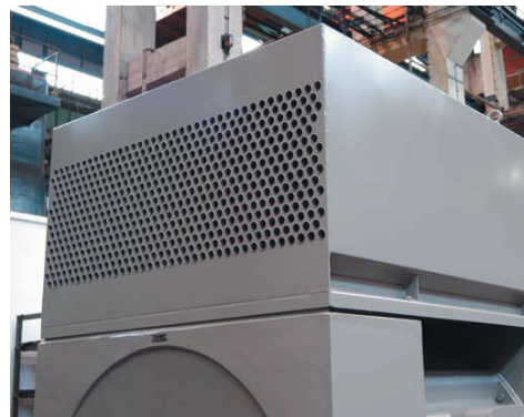
Closed cooling circuit (air-to-air)
