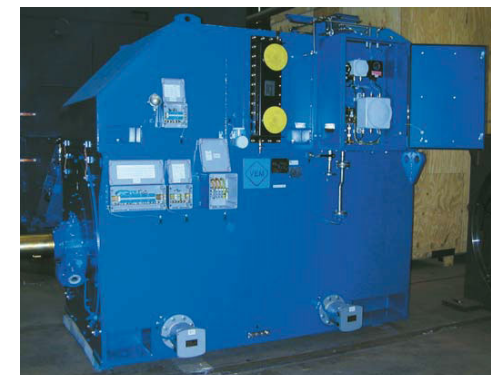
Synchronous motor, 3.5 MW extruder drive (EEx p)
