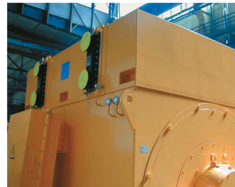
Closed cooling circuit (air-to-water)
