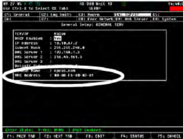
Figure 3 - MAC Address on TCP/IP Screen
