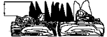
Figure 15 - Correct Flame Pattern With Control Knob Set to High Flame
