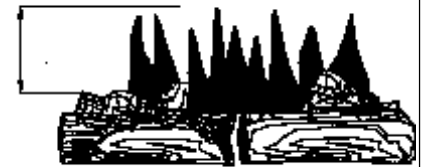
Figure 16 - Incorrect Flame Pattern With Control Knob Set to High Flame
