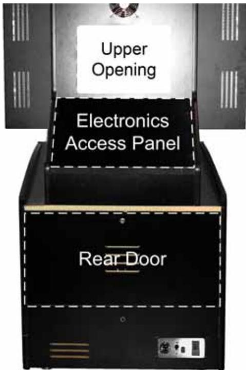
Use the access panels on the rear of the cabinet to service internal components.
