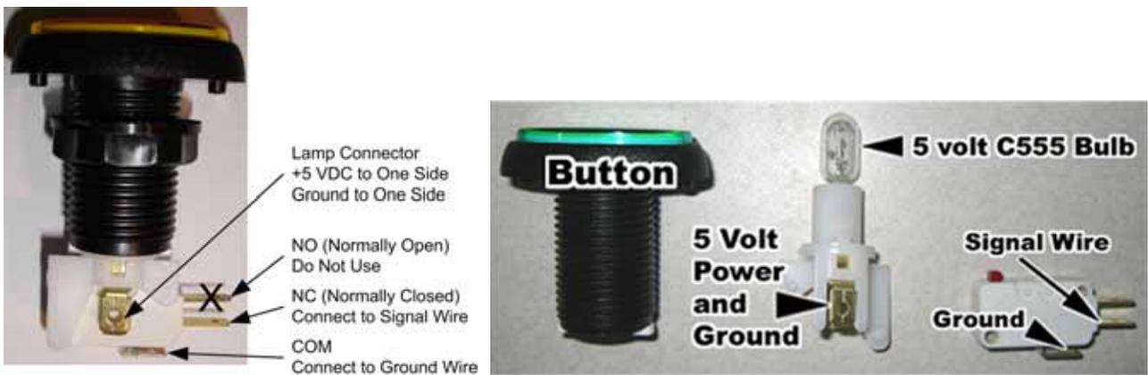
*Figure 12. Replacing Button Components*
