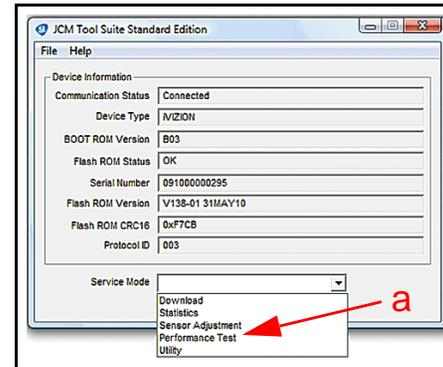
**Figure 7** Typical Connected iVIZION JCM Tool Suite Screen
