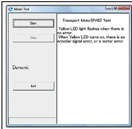
**Figure 9** Typical iVIZION Transport Motor Test Screen
