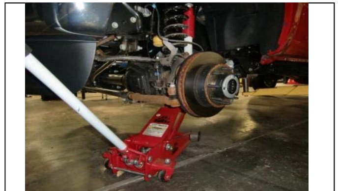
Support front axle with floor jack(s).
