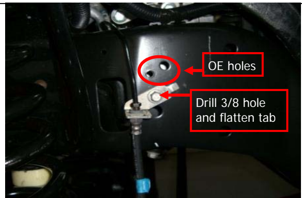
Shown, pass. side new 3/8 brake line hole location.
