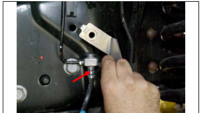
(11-up) models replace OE bracket with new drop bracket.
