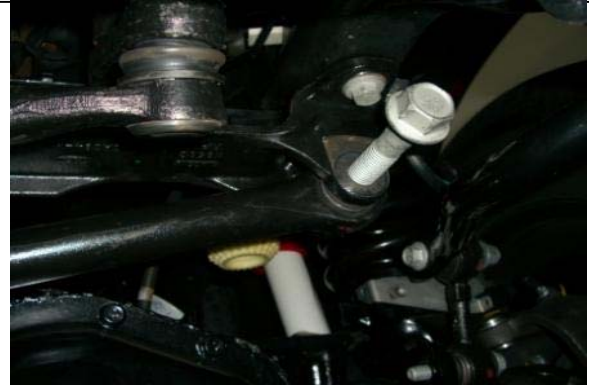
Remove upper track bar hardware and disconnect at frame.
