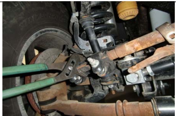
Adjust collar to straighten steering wheel
