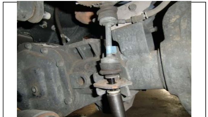
Disconnect both front sway bar end links
