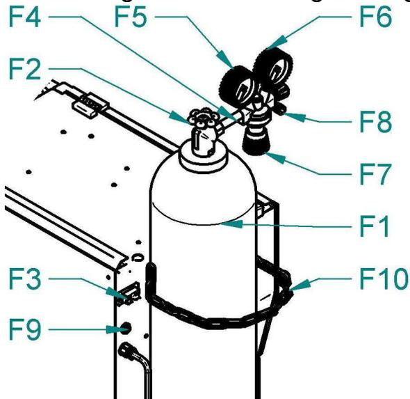
Fig. 7 – Gas fitting. The picture is just for illustration. The portable PEGAS 250/320 MIG MAN are not equipped to support the gas cylinders. The gas cylinders must be well fitted in another gadget in accordance with the appropriate safety rules.
