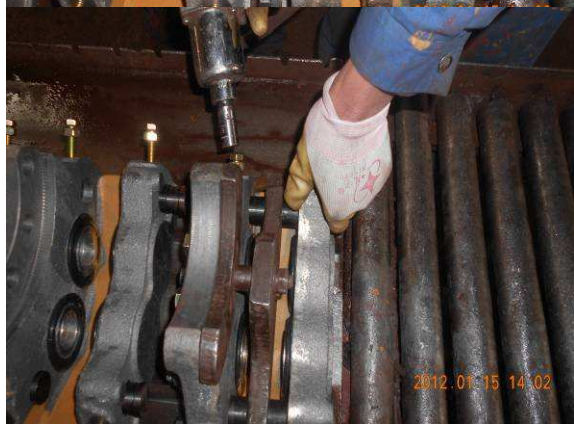
12. Assemble the pin shaft and tightening bolt.
