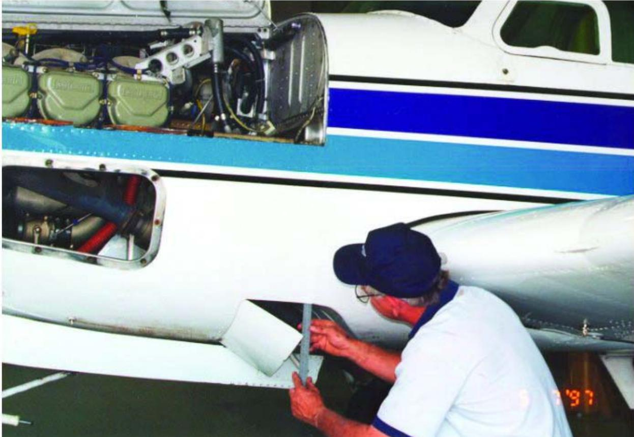
1. Verify that equipment such as add-on accessories and their associated hardware does not restrict cowl inlet, cowl outlet, and air flow through the cooling fins.
