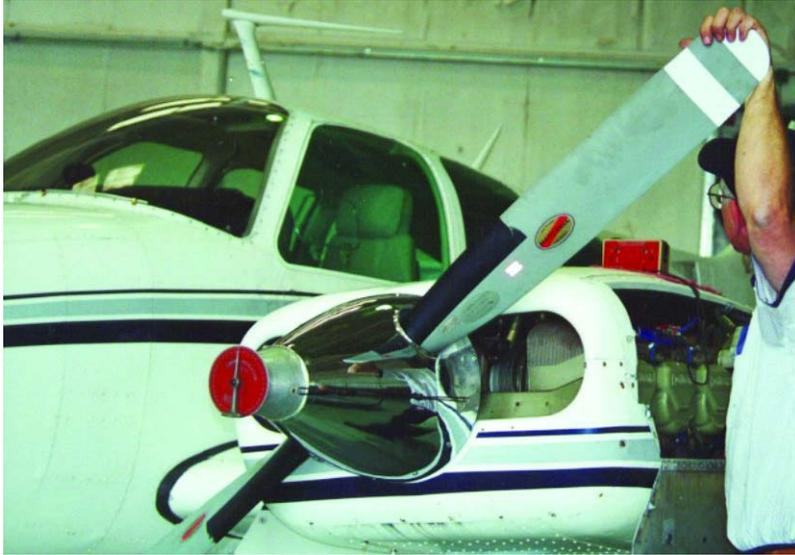
Incorrect magneto to engine timing can cause elevated cylinder head temperatures. Maintain and adjust magnetos in accordance with the engine and magneto service instructions. Inspect the ignition harness and spark plugs and replace if needed.
