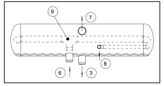
Figure 3 - Liquid Separator
