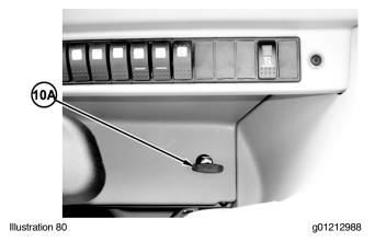
To connect the trailer, raise the hitch off the safety hooks and pull safety hook release cable (10A). Once the cable has been pulled, lower the hitch until the hook is at the required height in order to lift the tow eye. Reverse the machine with assistance or by using the hitch mirror until the hook is under the center of the tow eye. Raise the hitch until the safety hooks are engaged. If necessary, connect the trailer brakes. The machine is ready for towing.
