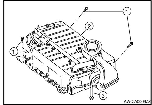
20. If necessary, remove the following components from the HV battery assembly.
