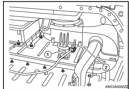
7. Remove the lock (1) from the RH cover (6) on the HV battery assembly (7) using the service plug grip (2).
