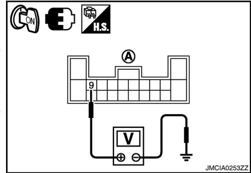
**4. CHECK HARNESS AND CONNECTOR (BATTERY COOLING BLOWER - BATTERY SMART UNIT)**
