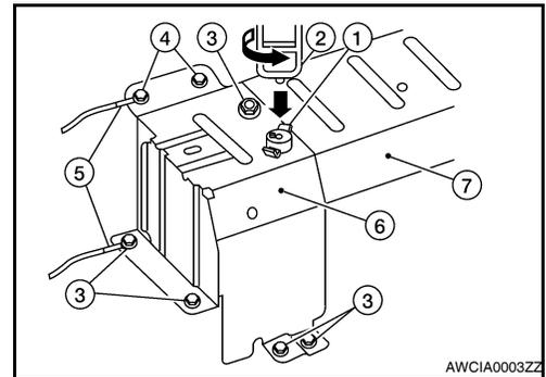
10. Remove the terminal cover and 12 volt terminal nut (1), then remove the terminal cable (2) and 12 volt harness from the HV battery assembly.
