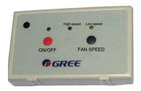
When pressing the ON/OFF button of the wireless remote control, the unit will run at high-speed. When pressing the FAN SPEED button of control panel, the unit will be switched over from the high-speed running to the low-speed running. Press ON/OFF button again to turn off the unit.
