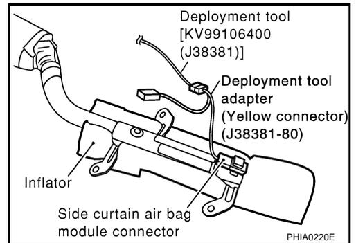
3. Put the inflator connected with the deployment tool [SST: KV99106400 (J38381)] into a tire without a wheel.
