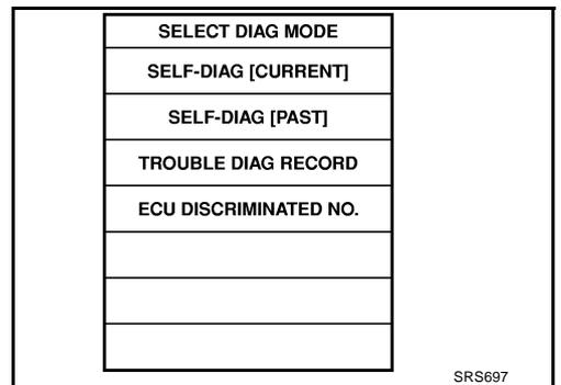
7. If no malfunction is detected on "SELF-DIAG [CURRENT]", repair of SRS is completed. Go to step 8.
