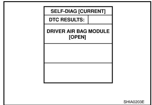
If no malfunction is detected on "SELF-DIAG [CURRENT]" even though malfunction is detected in "SRS Operation Check", check the battery voltage. If the battery voltage is less than 9V, charge or replace the battery. [SRS-23, "DIAGNOSTIC PROCEDURE 3"](#). If the battery voltage is OK, go to [SRS-26, "DIAGNOSTIC PROCEDURE 4 \(CONTINUED FROM DIAGNOSTIC PROCEDURE 2\)"](#) diagnose the following cases:
