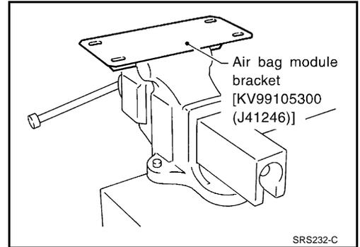
2. Match the hole in air bag module bracket (held in vise) and front passenger air bag module and fix them with one bolt [M8 x 25-30mm (0.98 - 1.18in)].
