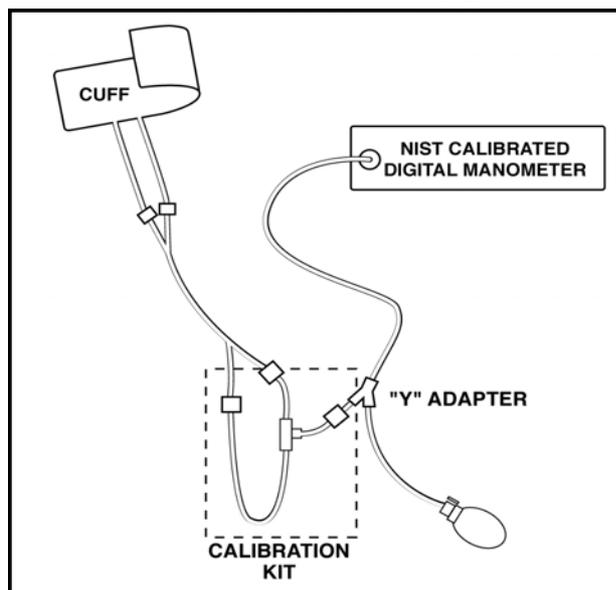
**Leak Test Setup**
