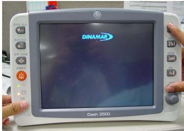
Continue to hold the "Main" and "Print" hardkeys until the monitor displays the logo on the screen. At this point the download process will automatically resume.
