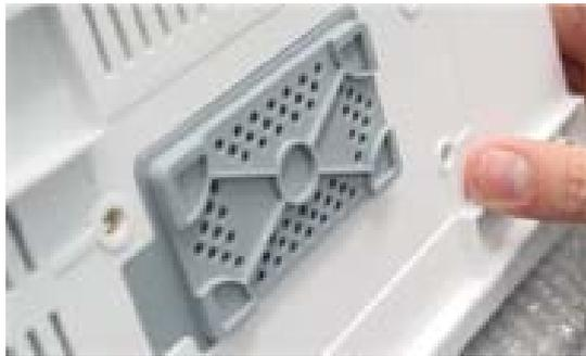
3. Release the lock and then take out the battery and wires.
