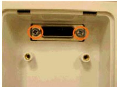
4. Connect the network module board into the port
