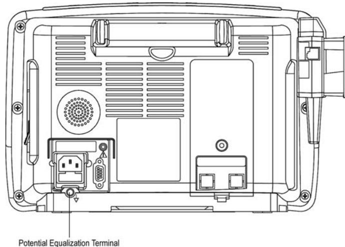
**Rear View of Monitor with Safety Connection Exposed**
