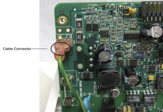
3. Remove the four screws and replace the DC2DC PWA.
