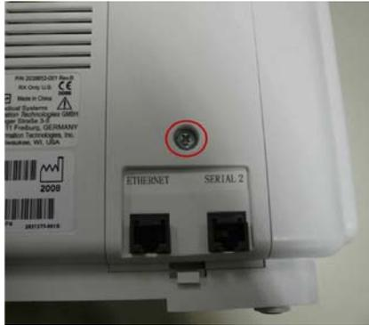
3. If the monitor is the old version, replace the port's two screws into new screw-locks (PN 2038990-001), with the 5mm hexagonal socket wrench.
