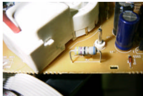
Correct type Metal oxide resistor PN: 11347020575 47 Ohm, ½ W
